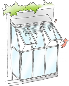
AUTOMATED WINDOW OPENING & SHADING TO CONSERVATORY
